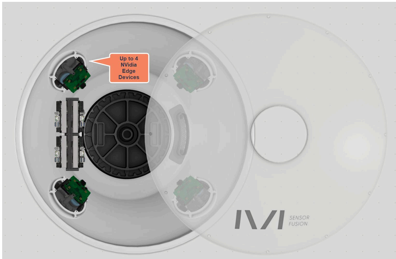
Figure 4. Internal view of the Minerva Platform showing the location of up to 4 edge computing devices
