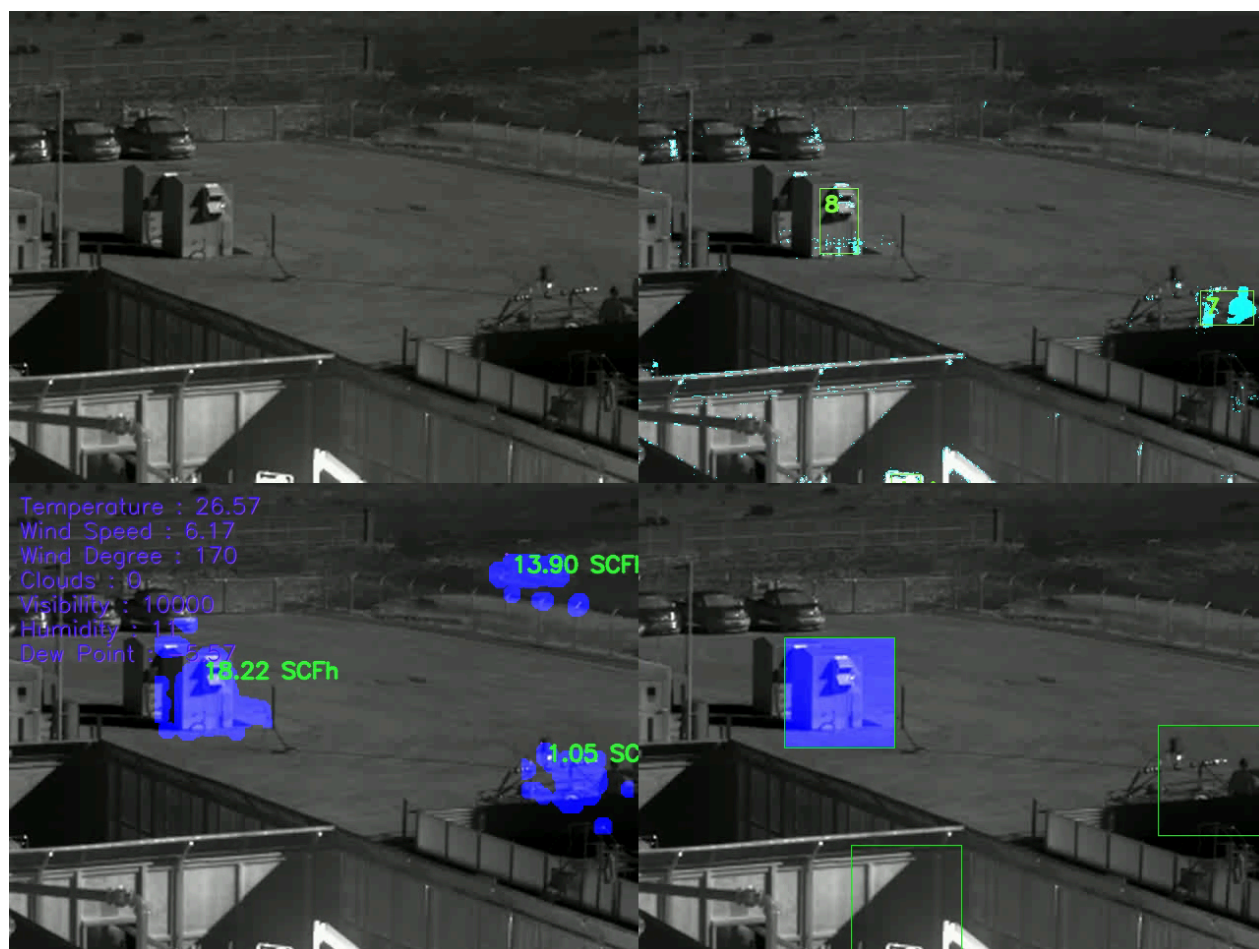
Figure 24. Controlled release testing 3 OGI video footage of the 80m test showing the CleanConnect LeakFinder's ability to localize an emission down to a component scale.
