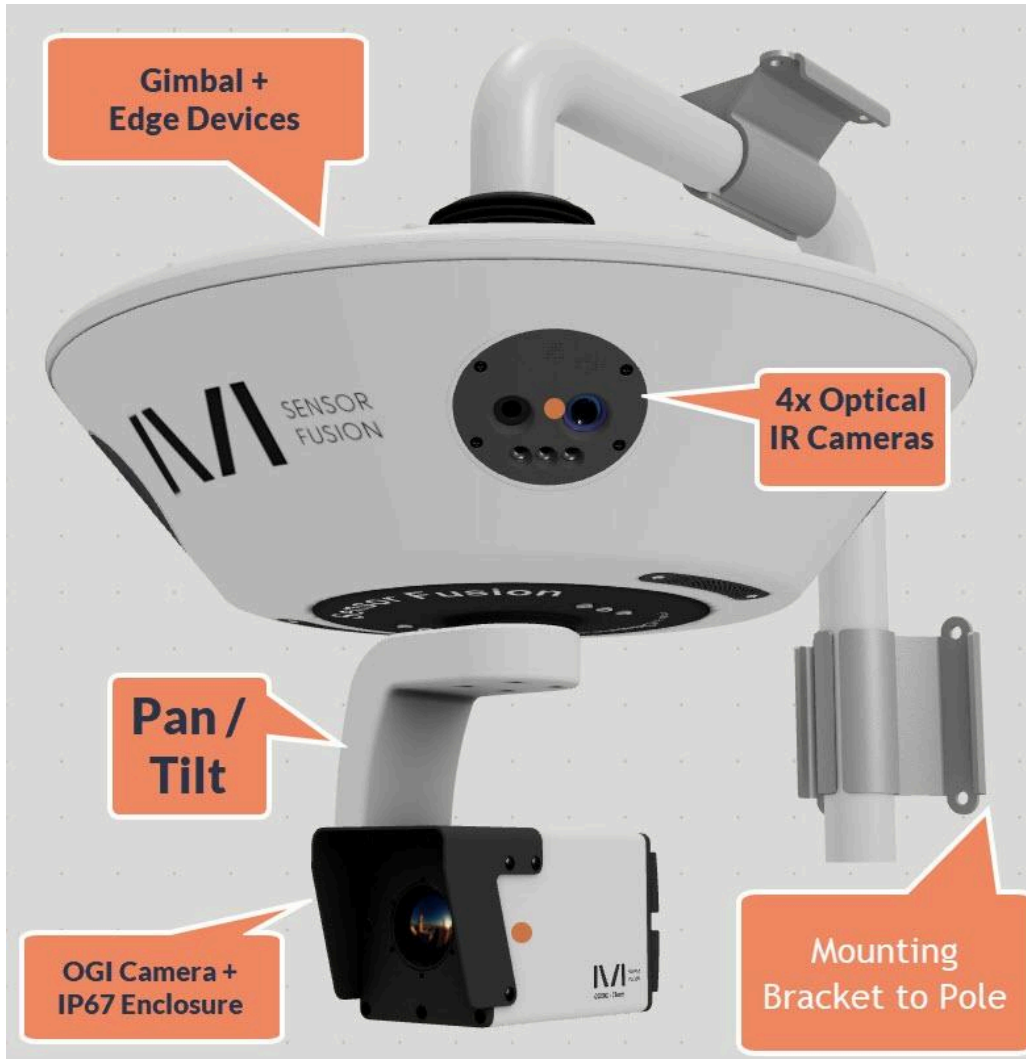
Figure 3. External view of the Minerva Platform, the primary physical component of the CleanConnect LeakFinder system.
